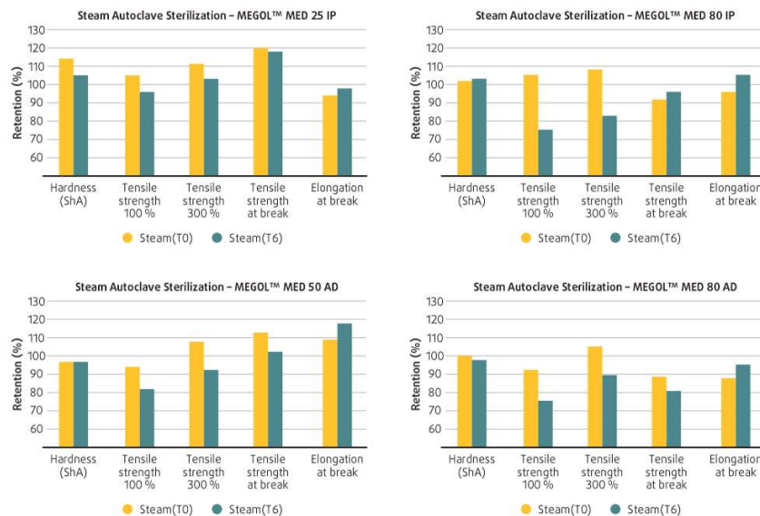
Figure 32–35: Effect of steam autoclave sterilization on property retention and yellowness index variation of MEGOL™ MED immediately after sterilization (T0) and after 6 months storage (T6).
